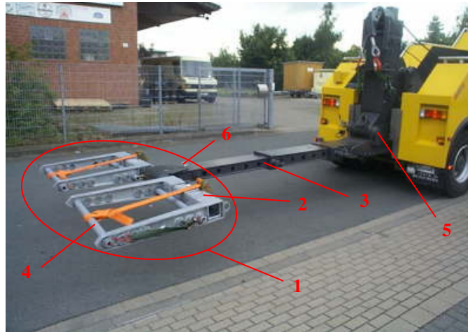
Fig. 2: underlift with mounted lift fork 1
